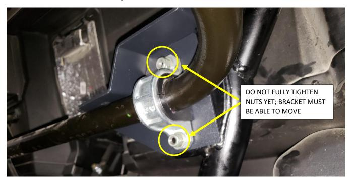
Figure 17 - Driver Side Sway Bar Nuts/Bolts with Air Tank Bracket Inserted
