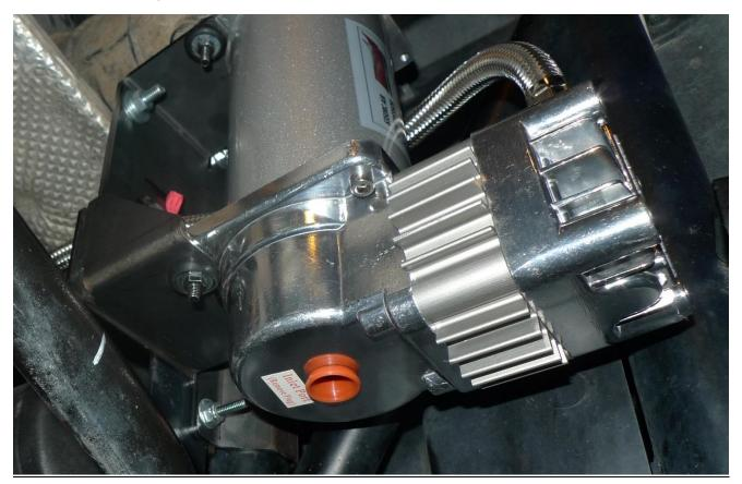
Figure 23 - Air Compressor Installed to Bracket
