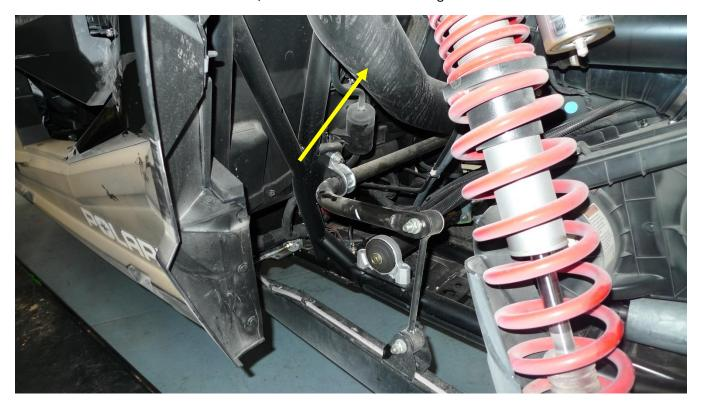
Figure 11 - Drive Belt Cooling Tubing, to Remove
