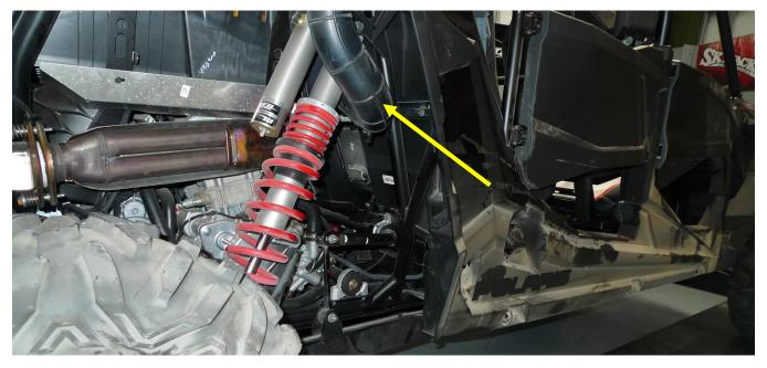
Figure 12 - Air Intake Tubing, to Remove
