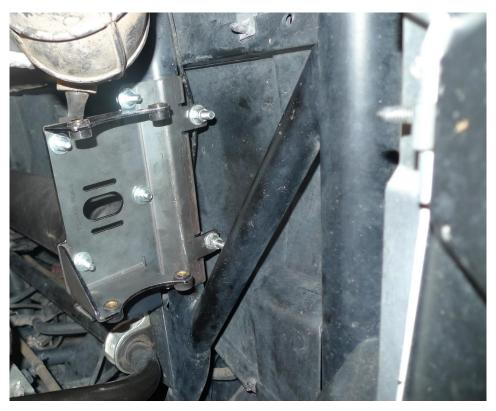
Figure 18 - Air Compressor Bracket Installed on Frame
