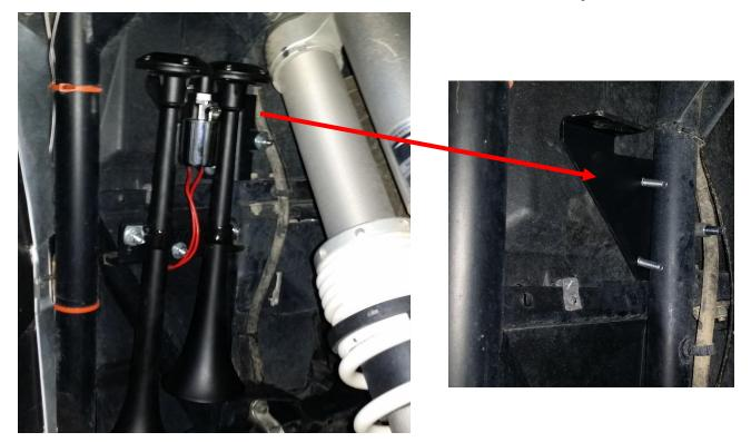
Figure 28 - Air Horn Installed to Brackets and Frame
