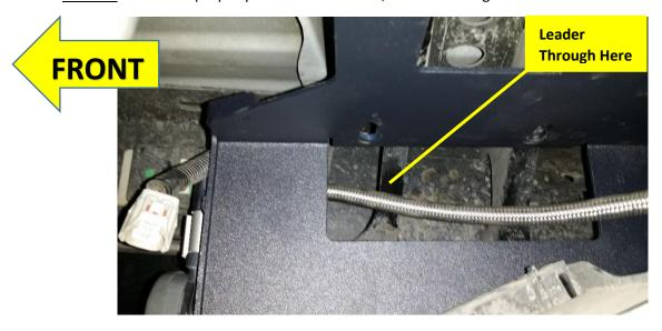
Figure 10 - Compressor Leader Hose Routing
