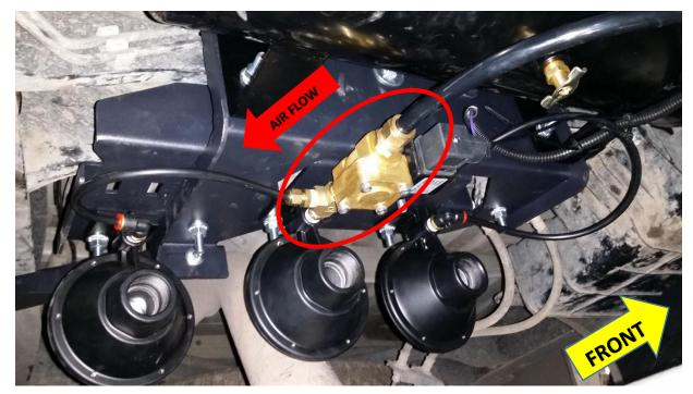
Figure 22 – Air Horn Drivers and Solenoid Mounted with Air Tubing Connected (730 Shown)
