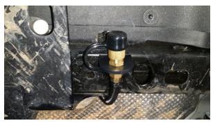
Figure 20 – Example of Air Coupler Mounted To Bumper
