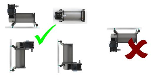
While the air compressor can be mounted in any position, Kleinn **DOES NOT** recommend mounting upside down as this <u>may cause</u> overheating & efficiency loss.
